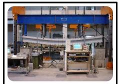
REFERENCE BEAM: PLASTIC DEFORMATION OF REBARS, LARGE DEFLECTION, FAILURE AT 2X68KN
